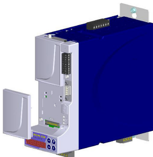
Figure 4.1: Remove the protective cover
