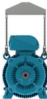
Figure 10 - Use of a spreader beam for lifting
