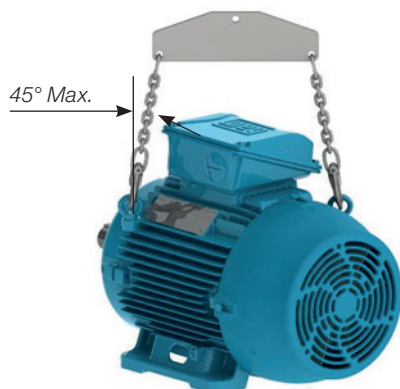
Figure 7 - Maximum resulting angle for motors with two or more lifting eyebolts
