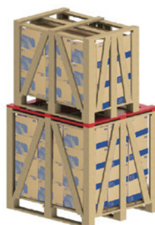
Figure 28 - Use of additional battens for stacking
