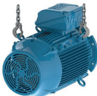
Figure 25 - Final result: motor placed in horizontal position
