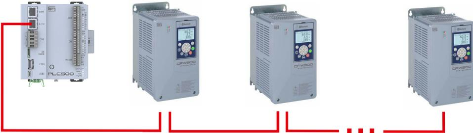
Figure 2.4: EtherCAT daisy-chain topology.
