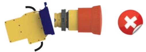
Flange NOT properly assembled on the pushbutton.
