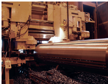
Machining radial slots in rotor forging.
