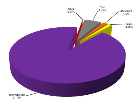
The materials used in the product range and the corresponding weight are disposed below, in *table 1*. The information about the constituent materials is referring to model EB05P-IP66.
