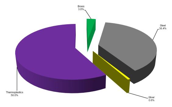
The materials used in the product range and the corresponding weight are disposed below, in *table 1*. The information about the constituent materials is referring to model BC10F-CSW.
