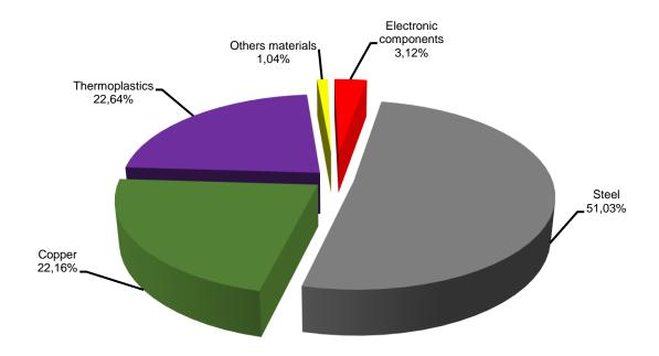
The materials used in the product range and the corresponding weight are disposed below, in *table 1*. The information about the constituent materials is referring to model RWM112-3-A4U112.
