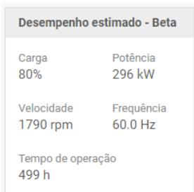
**Figure 9.18** - Beta Version of motor estimated performance – on the WEG IoT Platform screen.
