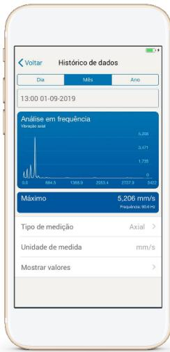
Figure 9.15 - Frequency vibration analysis - on the app screen.
