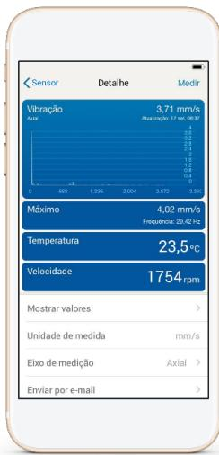
Figure 9.14 - Instant measurements on the app screen.
