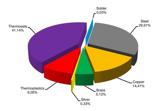
The materials used in the product range and the corresponding weight are disposed below, in *table 1*. The information about the constituent materials is referring to model DWB250N200-3DF.
