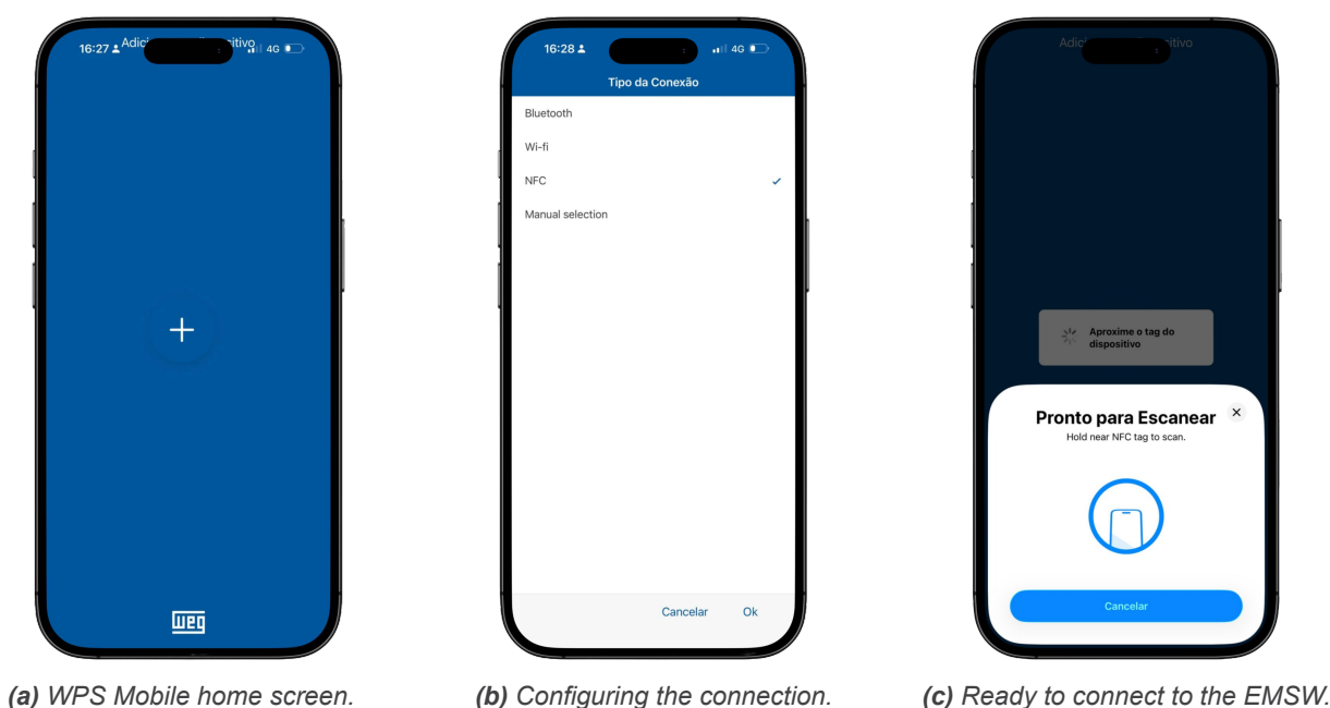
Figure 7.1: Steps for connecting WPS Mobile to the EMSW using NFC.
