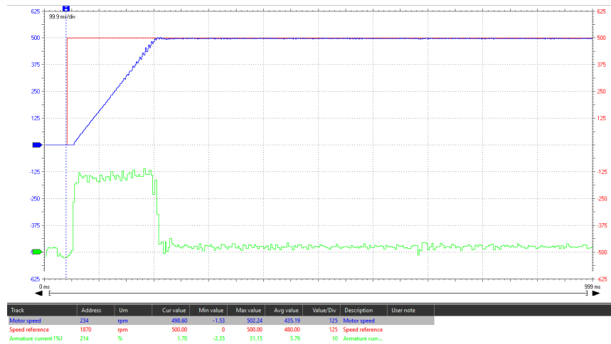
Figure 5-9: Speed reg P value too high, oscillations in armature current and speed
