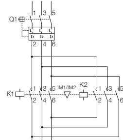
Note: 1) For reversing or star-delta starters, mount the contactors with screws.
