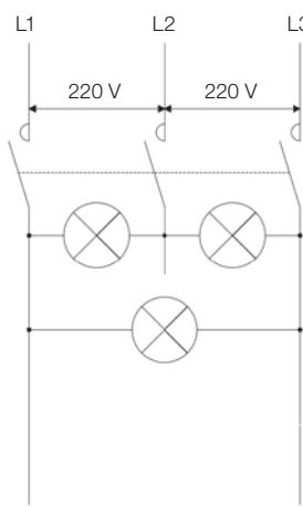
Three-phase circuit connected in delta
