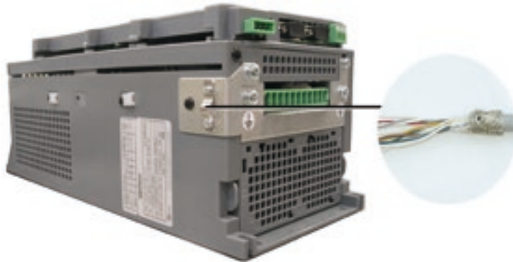
Figure 4.3.4: Connection of shielding (recommended)
