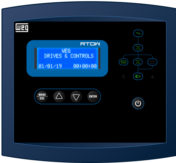
Figure 6.12: Rectifier HMI front view
