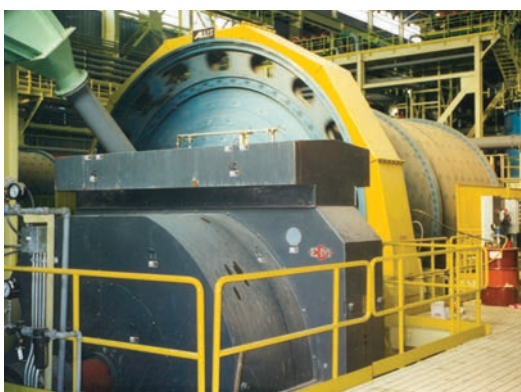
Metso Minerals – Minera Alumbra – Argentina 8000HP, 34 Poles, 3PH / 50 Hz / 6.6 kV
