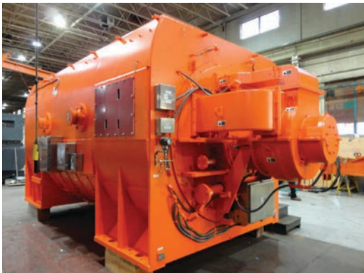
Mondi Paper – South Africa 56500 kVA, 2 Poles, 3PH / 50 Hz / 11.0 kV
