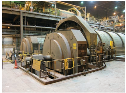
United Taconite LLC – Minnesota USA 3000HP, 44 Poles, 3PH / 60 Hz / 4.0 kV
