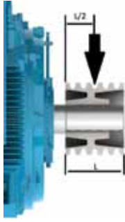
Figure 22 - Radial load position on shaft
