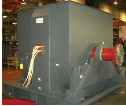
Baseplate with shipping cradle on flanged end.
