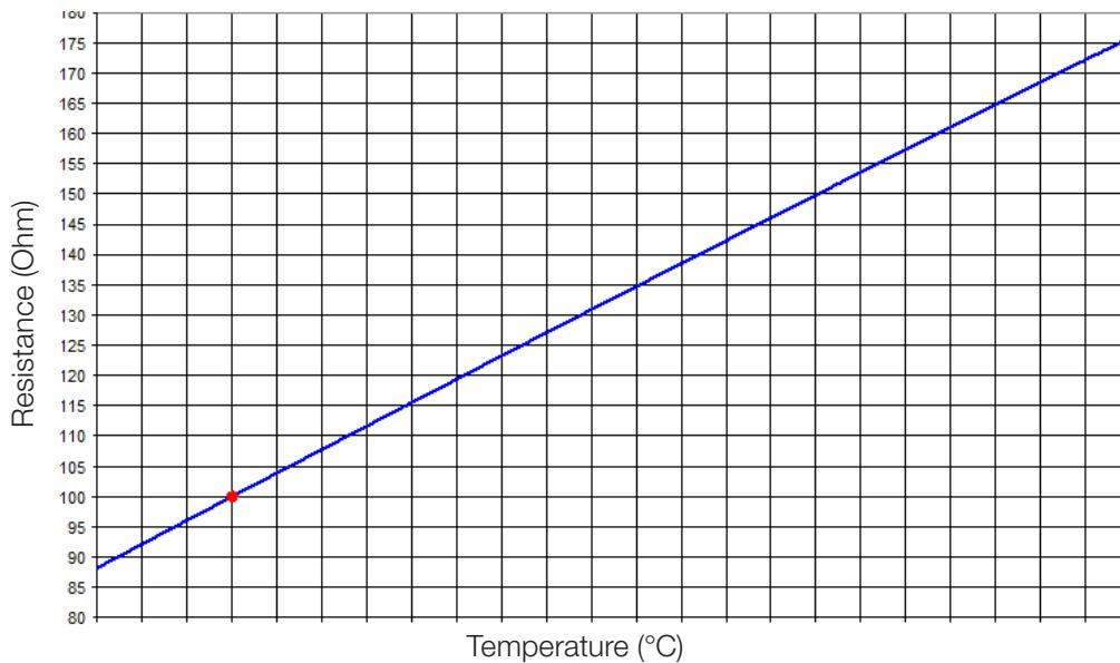
Figure 47 - Ohmic resistance of the Pt-100 x temperature
