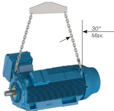
Figure 9 - Maximum resultant angle for horizontal HGF motors
