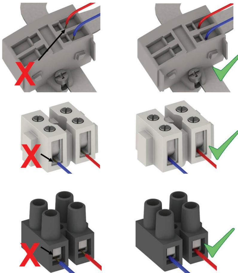
Figure 45 - Connection of the accessory cables to the connector.
