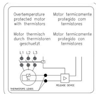
Figure 44 - Thermistor connection
