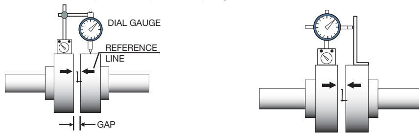
Figure 40 - Alignment with a dial gauge.
