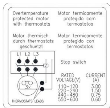
Figure 43 - Connection of the bimetal thermal protectors (thermostats)
