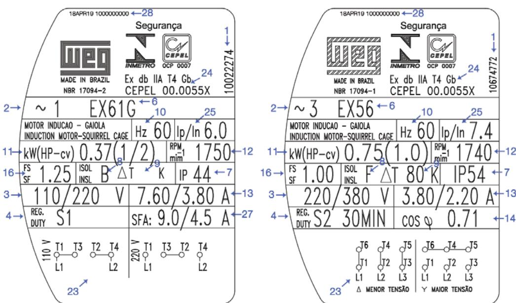
Figure 4 - Nameplate of the fuel pump motors.
