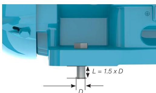
Figure 35 - Mounting system of a foot mounted motor
