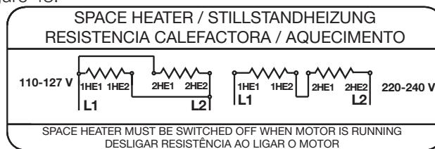
Figure 48 - Dual voltage space heater connection.
