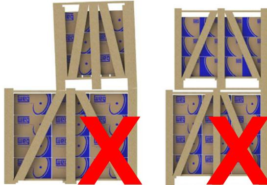
Figure 28 - Incorrect stacking
