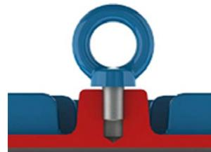
Figure 6 - Incorrect tightening of the eyebolt.
