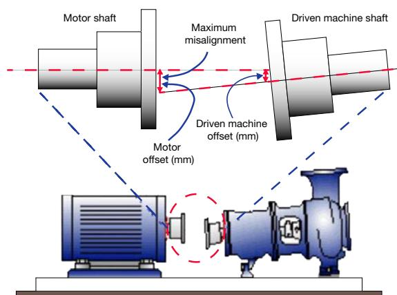
Figure 39 - Typical misalignment condition
