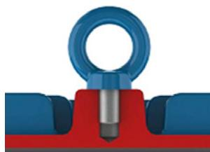
Figure 5 - Correct tightening of the eyebolt.
