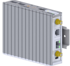
Figure 2.10: Gateway mounted on a DIN Rail
