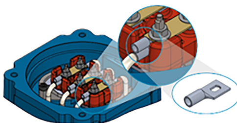
Figure 6.15: Representation of "Ex eb" terminal block with oblong holes on the terminal lug
