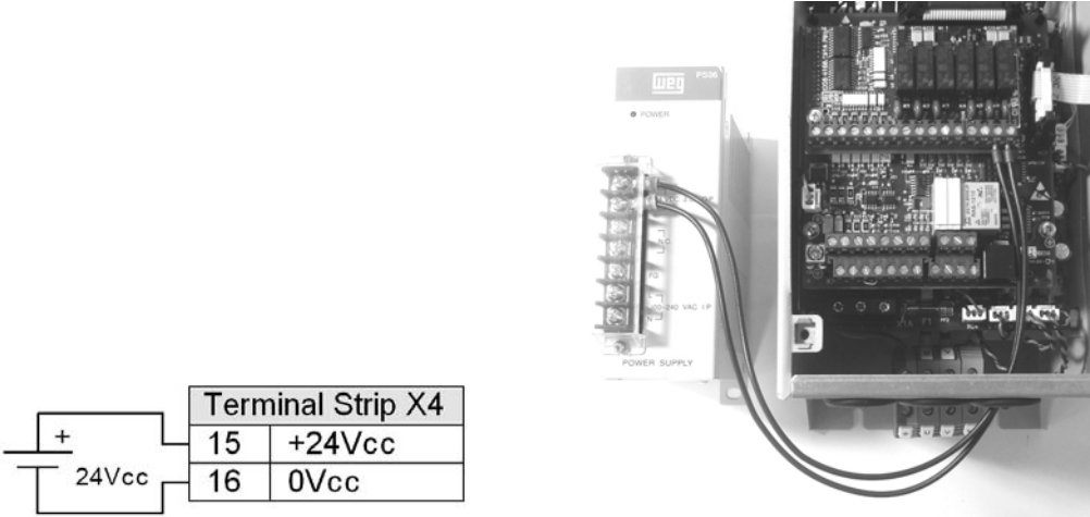
Figure 5.4: IOS6 board external power supply
