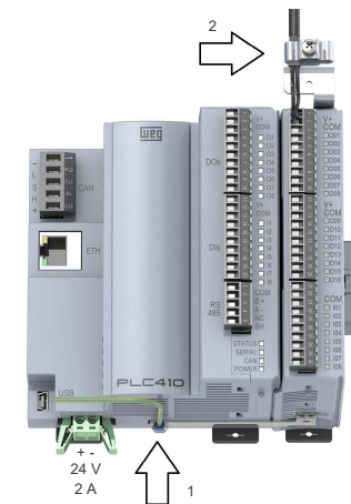
Figure A.3: PLC410 power supply and grounding
