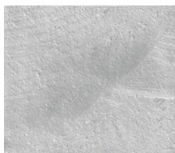
CSP 2 – Polimento com pedras 812,8 \mu\text{m}^1
