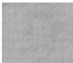
CSP 3 – Jateamento leve 965,2 \mu\text{m}^1
