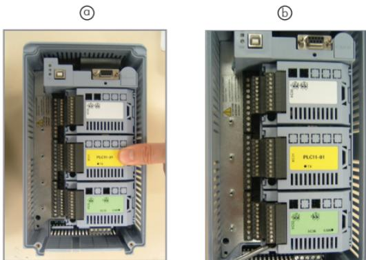
Figure 3: Installation of the accessory into slot
