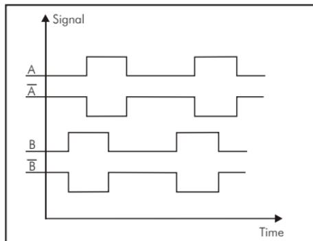
Figure 7: Standard phase of the encoder signals
