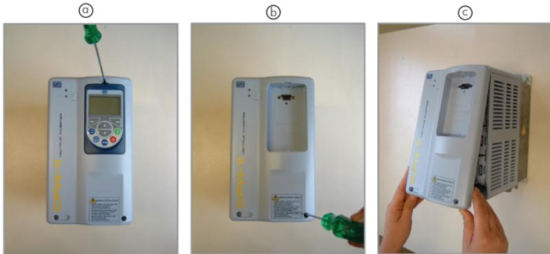
Figure 2: Removal of front cover
