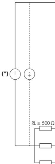
(\*) The internal 24Vdc power supply can be used by connecting XC30:9 to XC31:5 and XC31:4 to the load.
