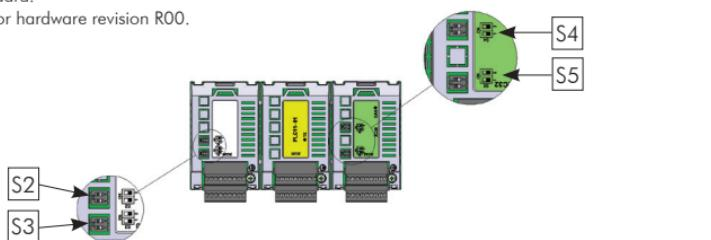
Figure 4: Location of the configuration switches
