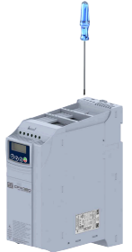
(c) Tighten the screws of the supply terminal of the CFW320 (Torque: 0.8 N/m) (c) Apriete los tornillos del borne de alimentación del CFW320 (Torque: 0.8 N/m) (c) Aperte os parafusos do borne de alimentação do CFW320 (Torque: 0,8 N/m)
