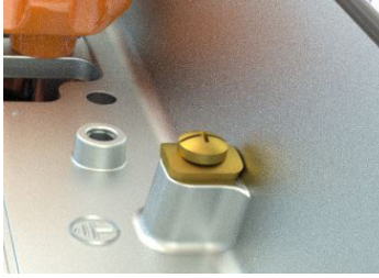
Figure 12 - Grounding terminal 71,W80,90L and W100L the terminal box Motor power supply leads are marked in accordance with IEC 60034-8 and are connected to a terminal block made from a polyester based resin BMC (Bulk Moulding Compound), duly reinforced with fibre glass.
