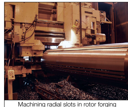
Machining radial slots in rotor forging
