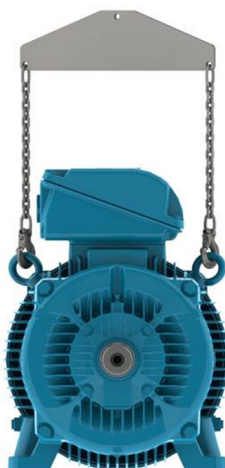
Figure 4.7: Use of a spreader beam for lifting
