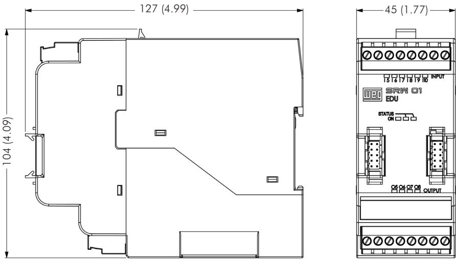
Figure 8.10 - Dimensions of the Expansion Digital Unit – EDU – mm (in)
