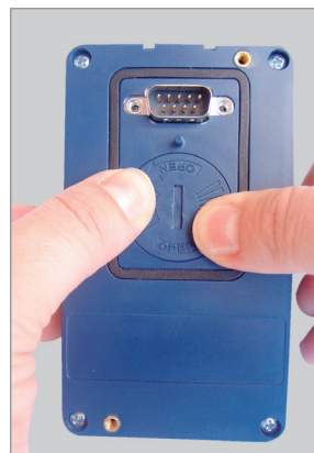
Put the cover back and rotate it clockwise
