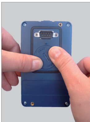
Press the cover and rotate it counterclockwise
