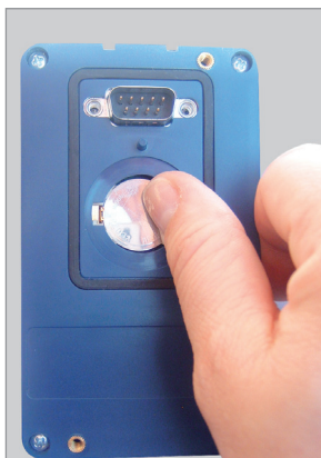
Press the battery for its insertion
