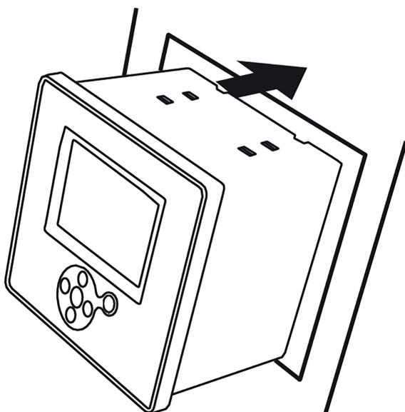
*Figure 2.1: Placing PFW03-M on the panel*
