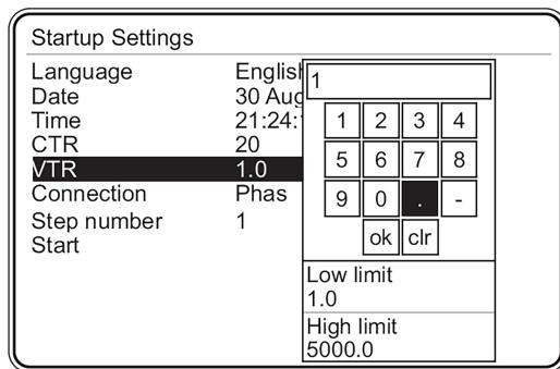
Figure 3.7: Voltage transformer ratio
