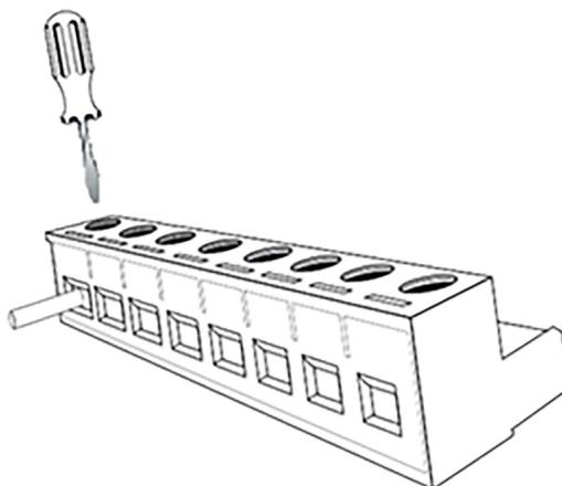
*Figure 2.5: Fixing the cable to the terminal block*
