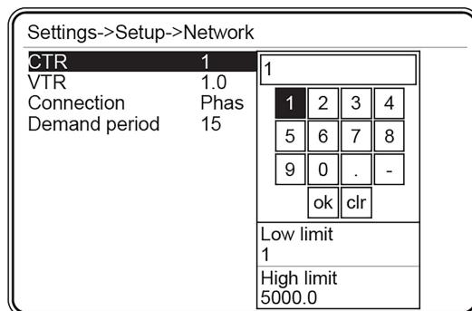
*Figure 3.17: Current transformer ratio setting*
