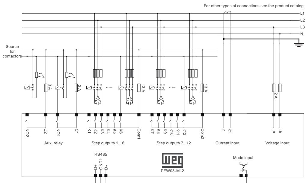
**Figure 2.6:** PFW03-M connection diagram (12 Steps)
