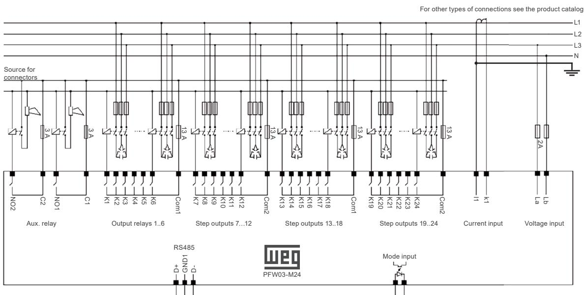
**Figure 2.7:** PFW03-M connection diagram (24 Steps)
