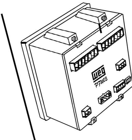
Figure 2.2: Securing PFW03-M
