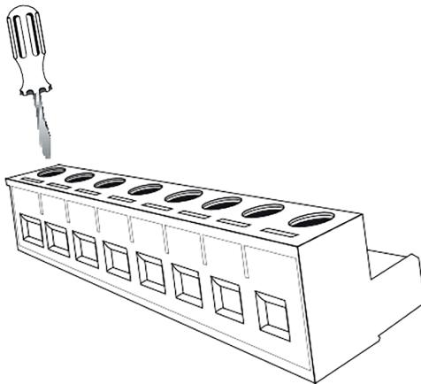
Figure 2.3: Loosening of the terminal screws
