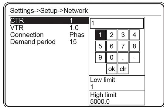
*Figure 3.18: Voltage transformer ratio setting*
