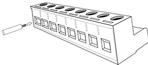
*Figure 2.4: Inserting cable into the terminal block*
