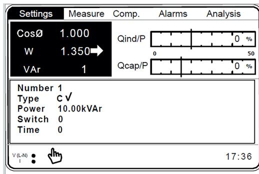
*Figure 3.34: Manual mod activated relay for PFW03-M24*
