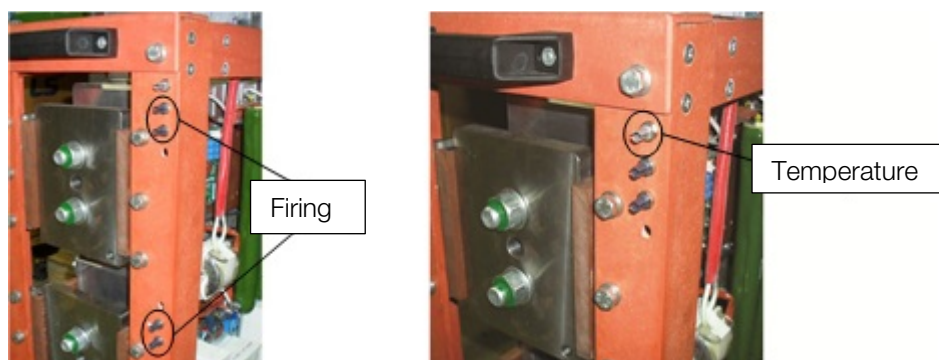
Figure 5.20: Firing and temperature Reading fiber optic cable connections – SSW7000
