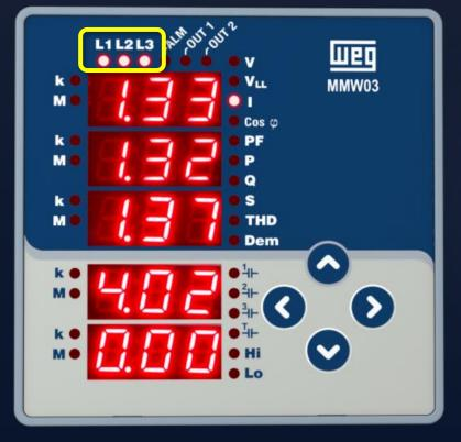
1) L1, L2, L3 flashing simultaneously and very slowly (1 per second):
