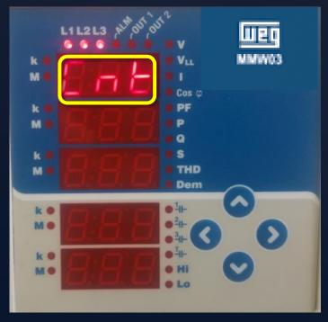
"On hour" Meter: The display shows the total hours that the equipment was energized. "Run hour" Meter: It shows the time the device performed the measurement. It is necessary that the signal inputs be fed by the three current phases and three voltage phases. "Int" Meter: It shows the number of energy interruptions on the equipment.
