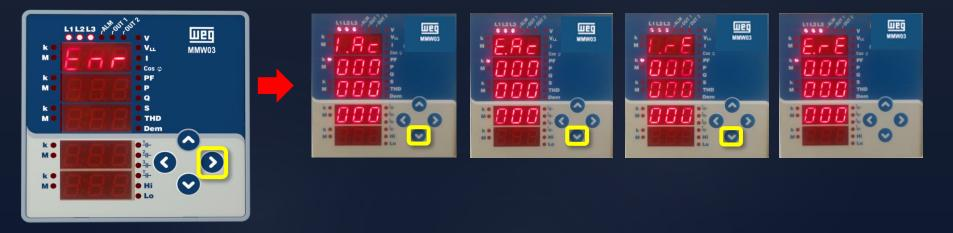
Preset value: In any menu on the device, press for at least 2 seconds and release. The menu will start flashing. Using the right arrow key, move the indicator to the digit you want to change. Enter the desired value using the up and down arrow keys. After entering the desired value, use the left arrow key to confirm the operation. Navigate through the menus to the storage field to save the preset value.
