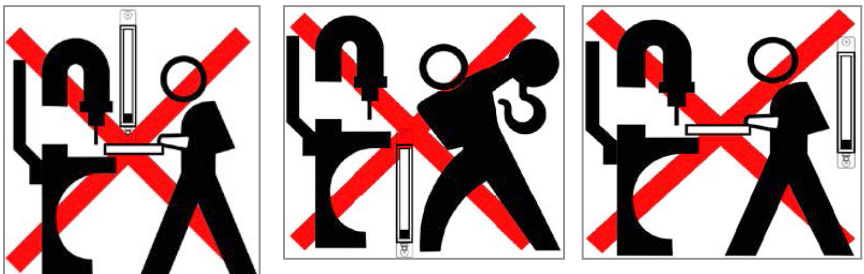
Figure 3.5: Incorrect positioning of the LGW300
