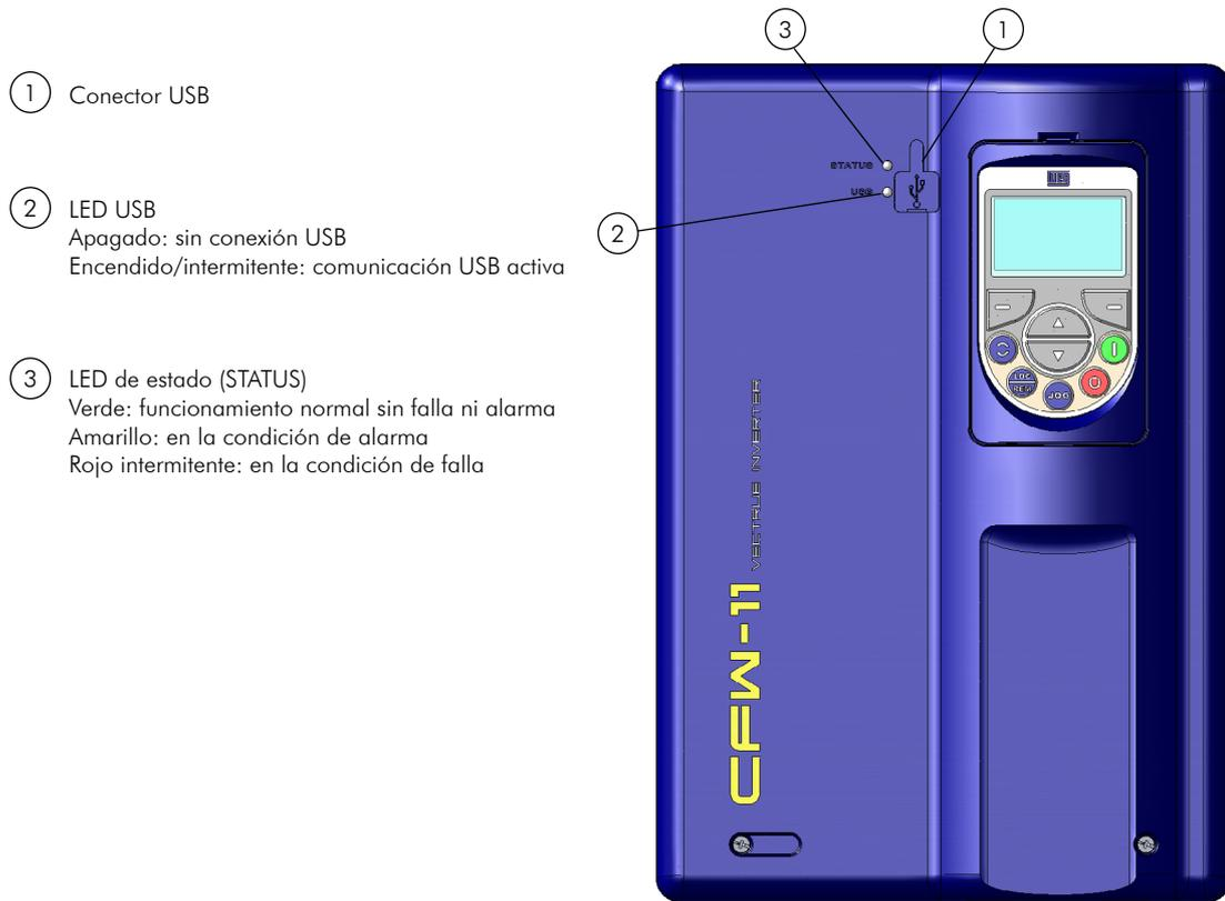
Figura 3.3: LEDs y conector USB
