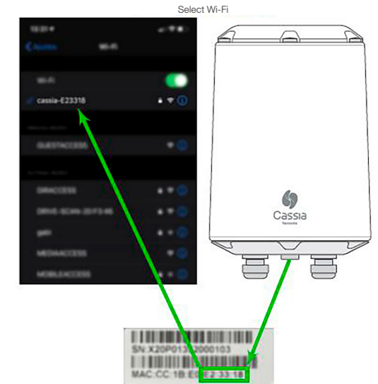
Figure 3.1: Location of the label with the MAC address used in the network SSID
