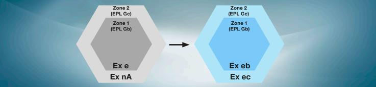
As a global supplier for the Oil & Gas market, WEG is in fully compliance with the new increased safety (Ex ec and Ex eb) marking, according to IEC/EN 60079-7:2015, including the product certificates IECEx, ATEX and INMETRO.
