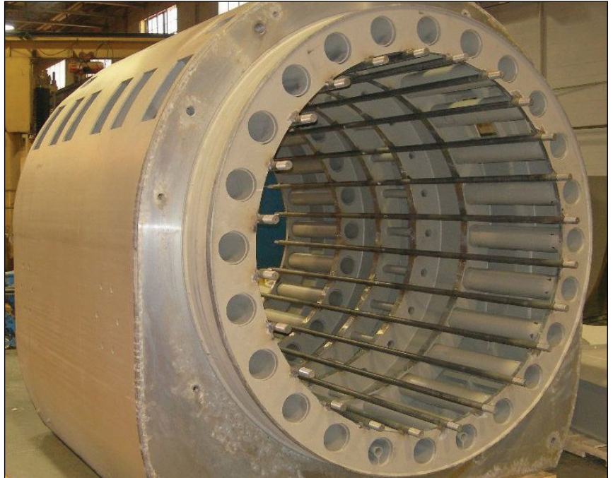
Stator frame center fabrication
