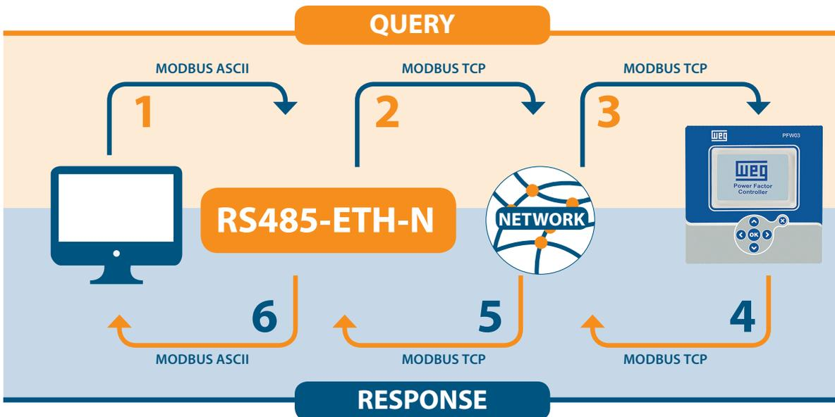
Figura 3.11: Client Mode Data Communication Scenario
