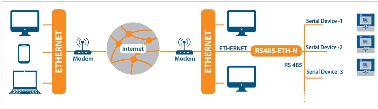
Figura 1.1: General Operating Principle of Server Mode
