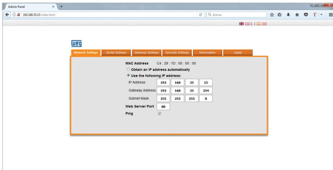
Figura 4.2: Web Interface Network Settings Tab
