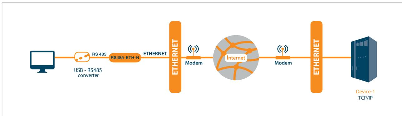
Figura 1.2: General Operating Principle of Client Mode
