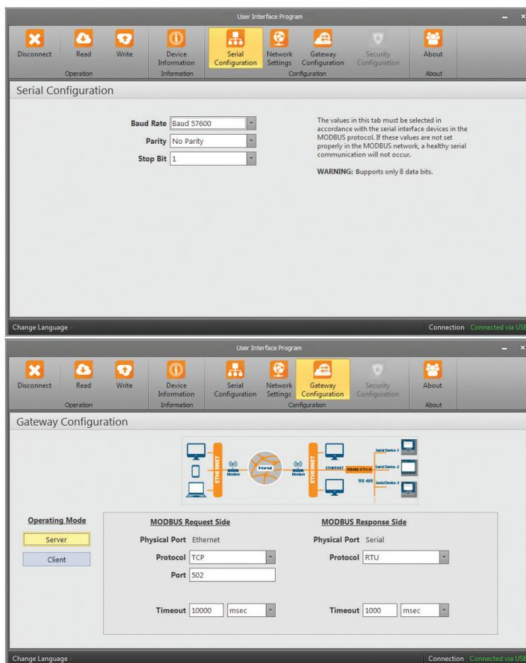
Figura 3.9: Server Mode Communication Example
