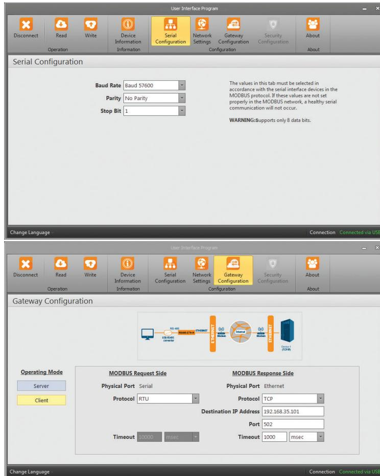
*Figura 3.12: Client Mode Communication Example*
