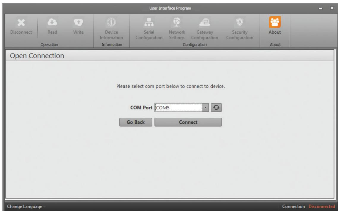
Figura 3.1: Virtual Com Port that RS485-ETH-N is connected
