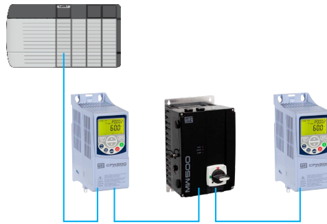
Figure 3.2: Daisy chain topology
