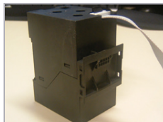
b) - Connection of the cable to the UMC
