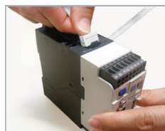
6 - Connection of the cable from the UMC to the Control Unit
