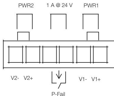
You can connect an alarm indicator, buzzer or other signaling equipment through the relay output. The relay opens if power input 1 or 2 fails ("Open" means if you connect relay output with an LED, the light would be off).
