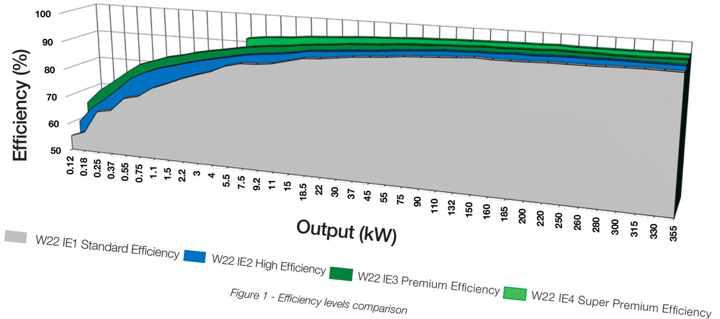
The comparative chart above shows the efficiency comparison between W22 4-pole motors with IE1, IE2, IE3 and the IE4 efficiency levels.
