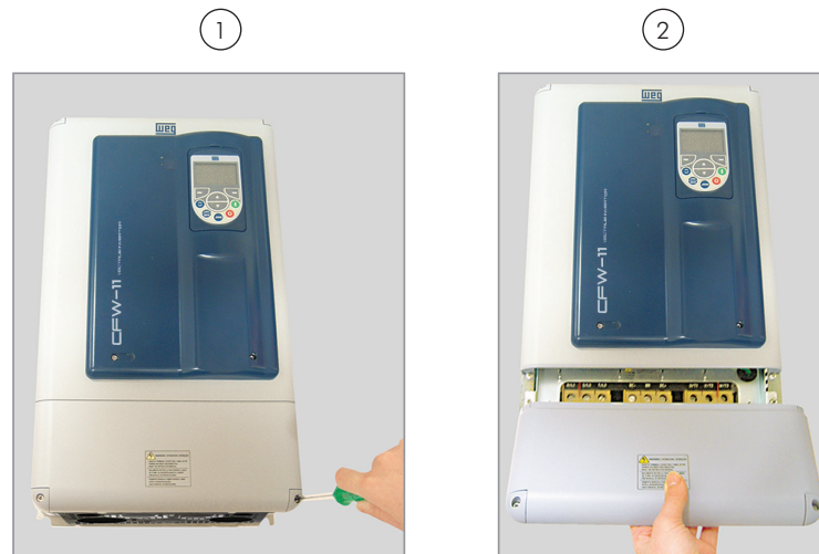
Figure 3.12 - Bottom front cover removal - frame sizes D and E
