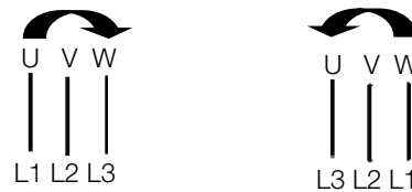
Figure 6.1: Phase Sequence (IEC60034-8)
