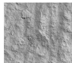
CSP 9 – Heavy scarifying 5435,6 µm*
