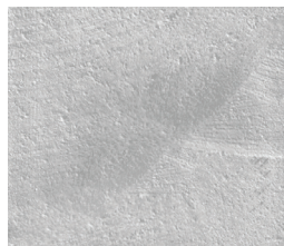
CSP 2 – Grinding 812,8 µm*
