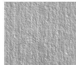
CSP 4 – Light scarifying 1270 µm*
