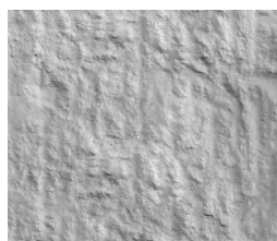
CSP 6 – Medium scarifying 3175 µm*
