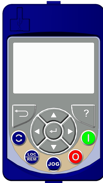
Figure 7.1: HMI Soft Keys.
