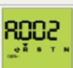
^ v   | 1. Communication Address value can be set between 1 and 247.<br>2. If Up button is pressed shortly, increases by 1. If pressed long, increases by 20.<br>3. If Down button is pressed shortly, decreases by 1. If pressed long, decreases by 20.                |
