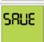
↩   | 1. Press Enter button if you want to save after setting. "SAVE" message appears and screen switches to measurement mode.<br>2. If you do not want to save, press Reset/ESC button. Then screen switched to measurement display right away. Data is not saved.   |
