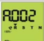
↩     | 1. If Enter is pressed once at Address view screen, screen is switched to Address setting mode.<br>2. Address blinks in one second interval.                                                                                                                    |
