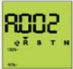
M×2   | 1. If Menu (M) button is pressed 2 times at measurement display, screen is switched to communication address view screen.                                                                                                                                       |
