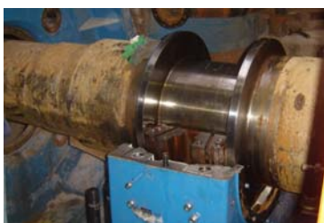
Figure 27: Corrosion on the shaft
